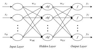
Figure 3. RBF neural network architecture of situation prediction.
