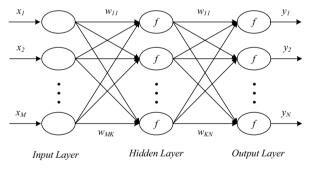
Figure 1. BP neural network architecture of situation prediction.
