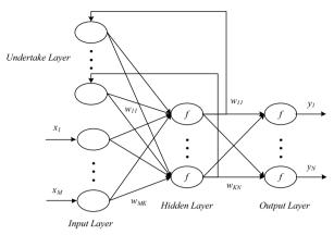
Figure 2. Elman neural network architecture of situation prediction.
