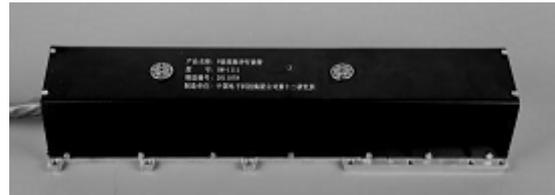
Fig.2 Photo of W band pulsed TWT for THz TWT cascade multiplier
