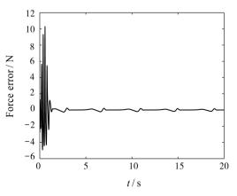
Fig. 2 Simulated responses of force tracking error at j = 1
