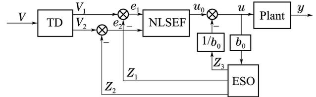
Fig. 3 The structure of ADRC algorithm
