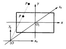
Fig. 1 Pinhole camera model
