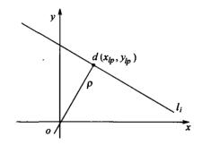
Fig. 2 Definition of line point in 2D image plane
