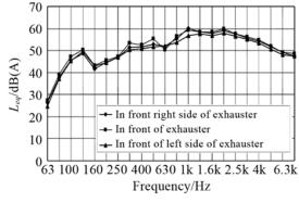
Fig.5 SPL at 3 measurement points in front of the exhauster
