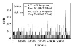
Fig.11 Time-domain specific roughness of the exhauster noise
