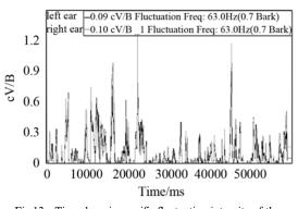
Fig.13 Time-domain specific fluctuation intensity of the exhauster noise
