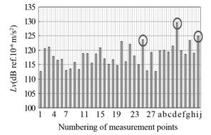
Fig.6 Vibration levels at 38 locations on different parts of the exhauster
