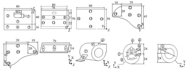
Fig.4 Locations for vibration measurements
