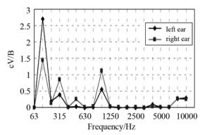
Fig.14 Specific fluctuation intensity spectrum of the exhauster noise
