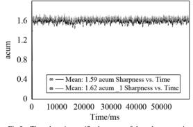
Fig.9 Time-domain specific sharpness of the exhauster noise
