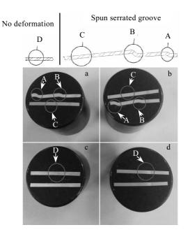
Fig.6 Inlayed specimens of serrated grooves on (a) and outside (b) the welded joint; undeformed parts inside (c) and outside (d) the welded joint zone
