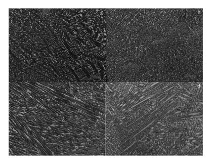
Fig.8 Microstructures of the as-welded joint: (a) area A, (b) area B, (c) area C, and (d) area D
