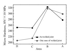
Fig.7 Micro-hardness distributions of the spun serrated groove
