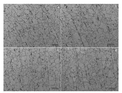
Fig.9 Microstructures of the outer zone of the welded joint: (a) area A, (b) area B, (c) area C, and (d) area D
