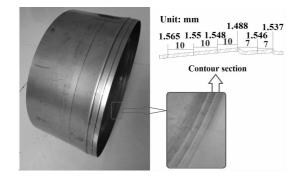
Fig.5 Spun part and its wall thickness distribution
