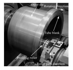
Fig.4 Assembly diagram of serrated groove spinning
