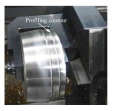
Fig.2 Profiling roller
