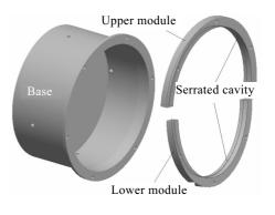
Fig.3 Serrated groove inner spinning dies
