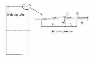
Fig.1 Section profile of the serrated groove
